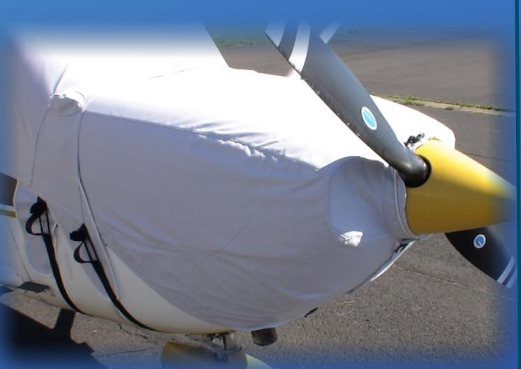
Two fixings are necessary to fit the Light cover of the C 152.
