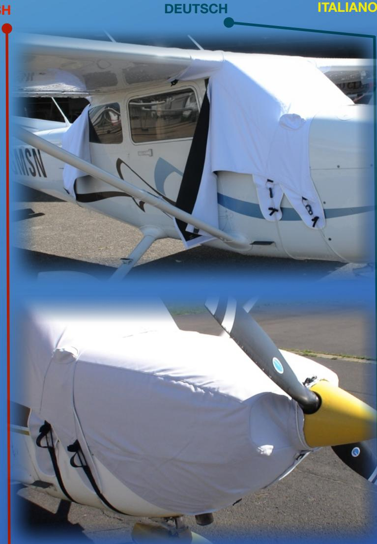
Several fixings are necessary to fit the cover of the C 172.
