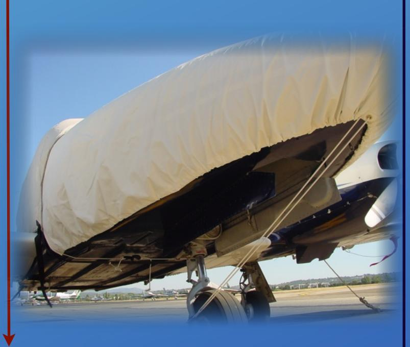
Several fixings are necessary to fit the cover of the SENECA .
