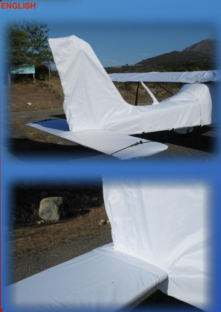
The wing covers are threaded over the wings covering the tips and are held onto the middle of the fuselage, they are joined between them by a Velcro fastening and two buckle clips, Hats cover the fuel caps and antennas.
