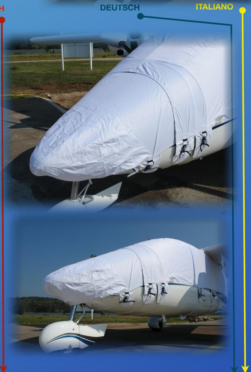
Several fixings are necessary to fit the cover of the P 68.
